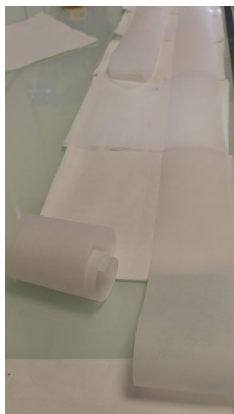
Figure 5 - Dismantling the Scale-X™ fixed-bed structure
